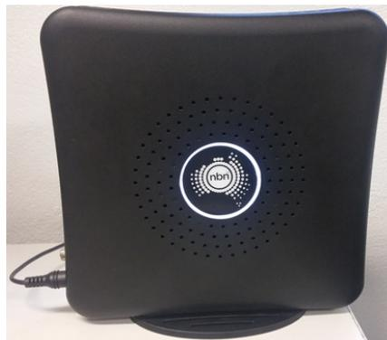
After locating the NTD in your home, connect it to your router by plugging a blue network cable into the “UNI-D 1” port as shown below. If “UNI-D 1” already has a cable connected, please contact customer service on 13 22 88 to find an alternate port.
