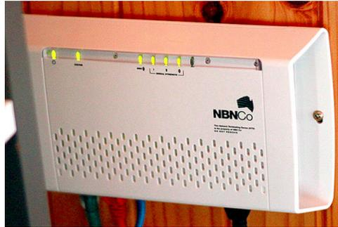
After locating the NTD in your home, connect it to your router by plugging a blue network cable into the “UNI-D 1” port as shown below. If “UNI-D 1” already has a cable connected, please contact customer service on 13 22 88 to find an alternate port.
