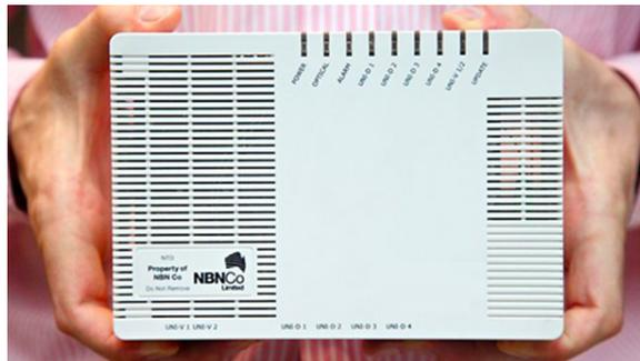
After locating the NTD, connect it to the router by plugging a blue network cable into the 'UNI-D 1' port as shown below. If 'UNI-D 1' already has a cable connected, please contact customer service on 13 22 88 to find an alternate port.
